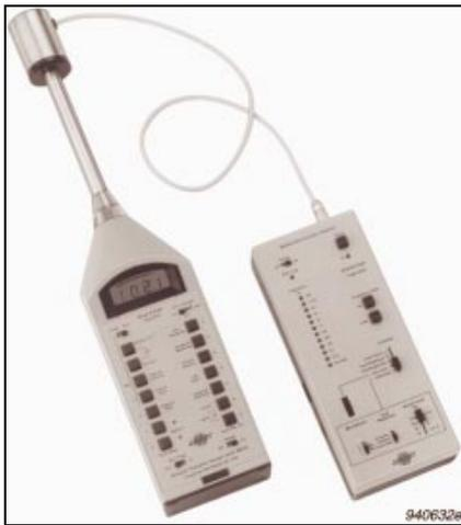
Fig 3 Checking and calibrating a sound level meter with Type 4226
